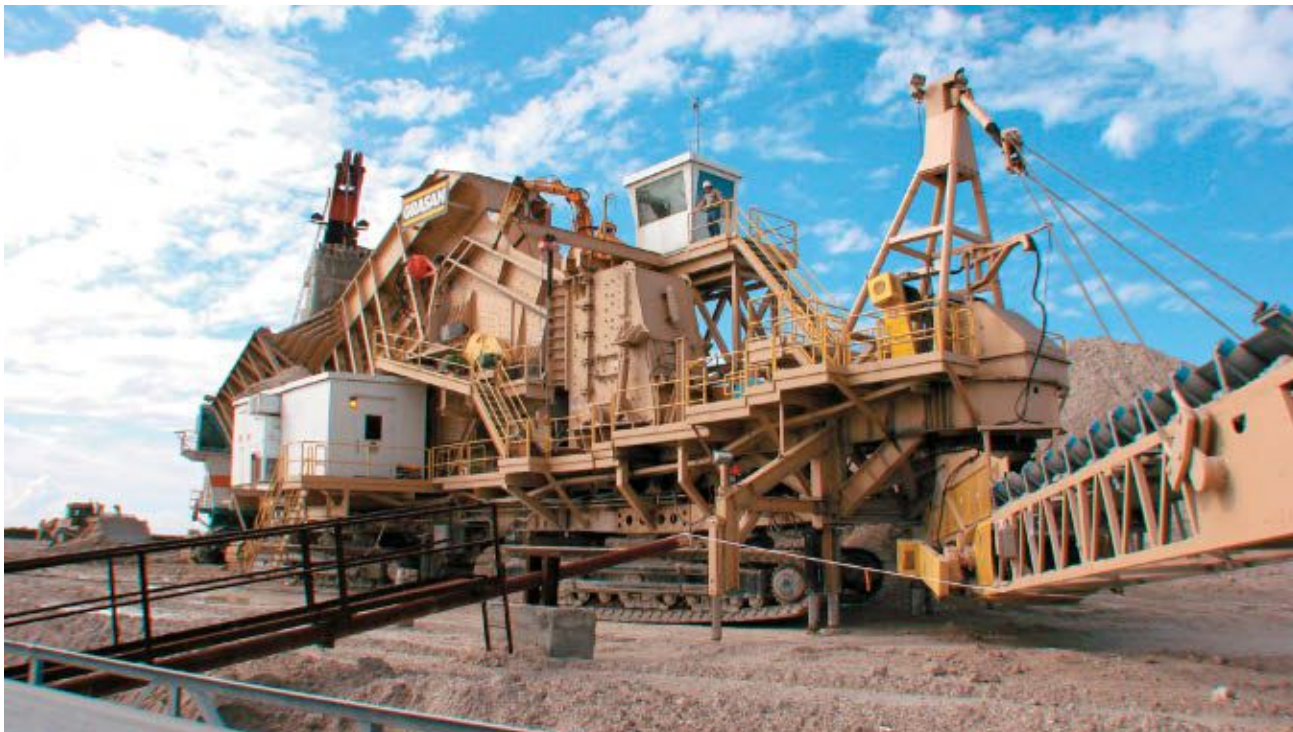
The Grasan 3,000-tph crushing plant is 47 ft. high, 39 ft. wide, 122 ft. long (183 ft. with discharge conveyor) and weighs 1.2 million lbs. It is mounted on two sets of custom-designed tracks with self-leveling stabilizer legs, can travel at ½ mph and can turn at various angles up to 90 degrees.
