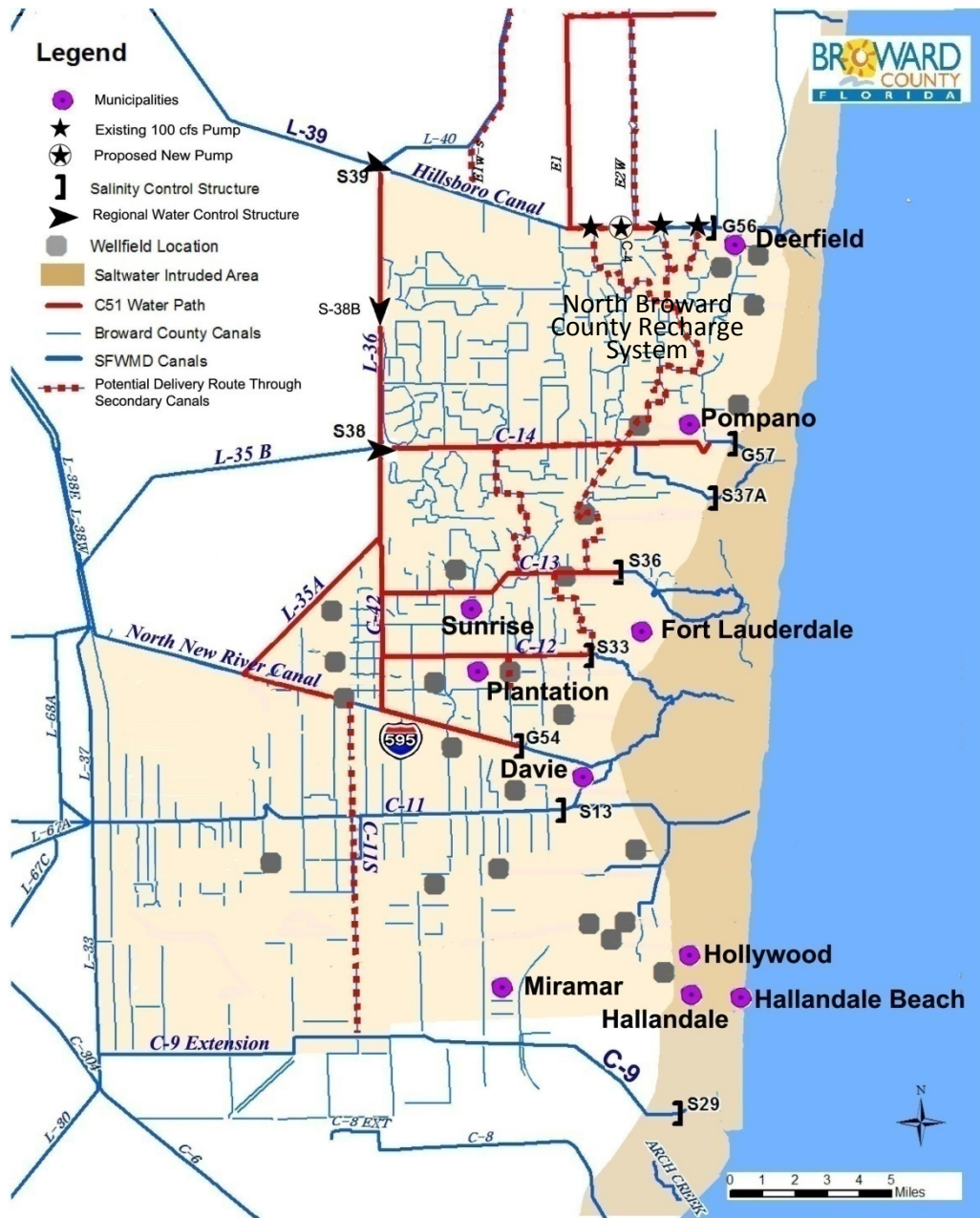
Figure 14. Locations of wellfields in Broward County that may benefit from additional water deliveries provided by the C-51 reservoir, and one proposed routing option (red and dotted lines) for providing these deliveries).
